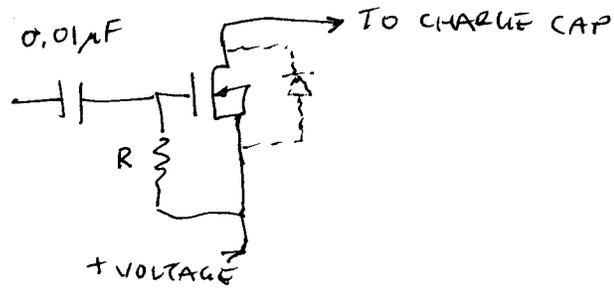
COUNT TAKES 264 20 $\mu$ S PULSES TO CHARGE CAP TO MAX VOLTAGE.
