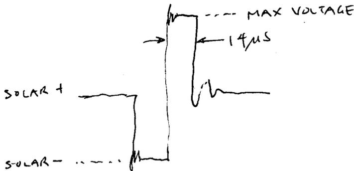
RINGING AFTER CHARGE ENDS IS SLOW - 210 KHZ. DON'T WANT TO LOSE ENERGY SHUDDING IT. HOWEVER, WITH SHUDDING HIGHER FREQ RIBBLG AT START OF PUMP + CHARGE - IT THREATENS GATE OF MOSFET.
