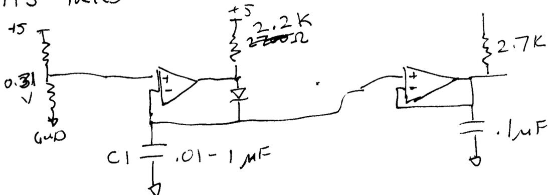
VOLTMETER READS 0.31V ACROSS C1, BUT IF CONNECT TO ADC, SEE NICE LIKE 3V. DITTO IF PUT VOLTAGE FOLLOWER AS SHOWN. LM393 USED. TRY LM358 INSTEAD.
