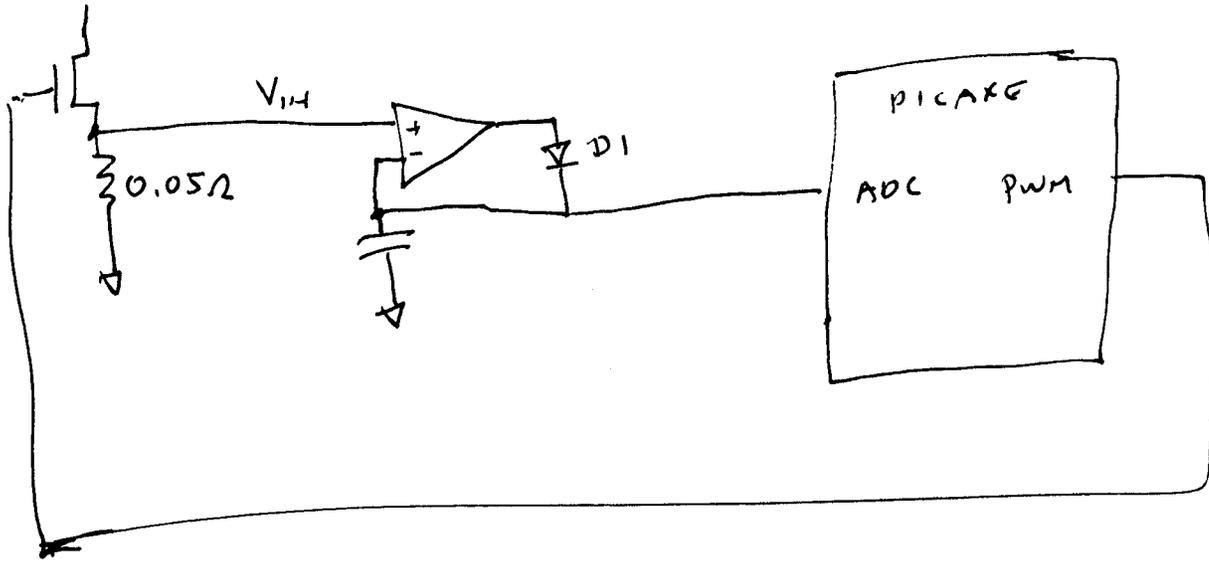
ANODE OF DI WOULD GO ABOVE CAPACITOR VOLTAGE, WHATEVER IT TAKES, TO CHARGE CAP TO VOLTAGE EQUAL TO  $V_{IN}$ .
