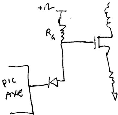
$$R_g = \frac{E}{I} = \frac{12V}{\frac{25mA}{24mA}} = \frac{1}{2} \times 10^3 = 500\Omega$$
